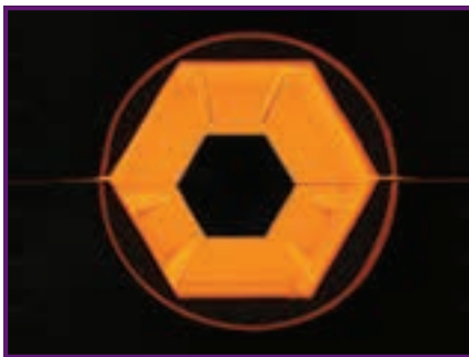
2 kW short wave halogen clamshell oven fitted with custom built short wave emitters. Used to heat wire/round tube up to 100mm in diameter.
