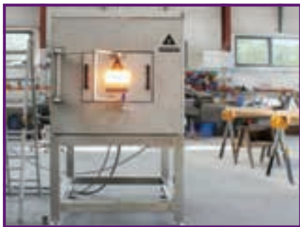
43 kW short wave halogen test oven fitted with custom built curved short wave emitters. Used as a high intensity material test oven in an aerospace application.
