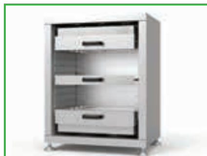
24 kW fast medium wave tungsten test oven fitted with quartz tungsten emitters model QTM. Used as a test platform for multiple materials in the automotive industry.
