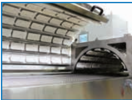
42 kW long wave ceramic conveyor oven fitted with white ceramic emitter model HTE. Used to cure foam on speaker housings.
